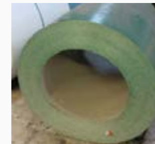
Ovalisation of a coil caused by poor storage practice.
